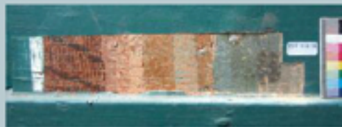
84. Stratigraphic study of the interior of one of the results of the partitions of the women's galleries. The paint layers have been exposed one by one with a surgical scalpel; this provides an image of all the different paint layers that are present, from the most recent one (on the left) to the earliest grey finishing layer (on the right).
